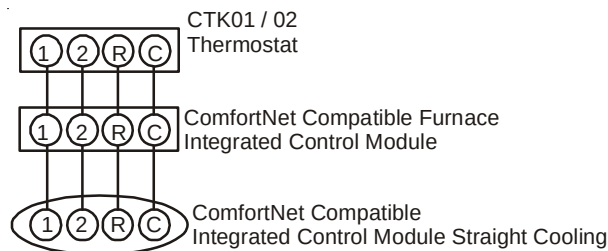
System Wiring using Four-Wires
